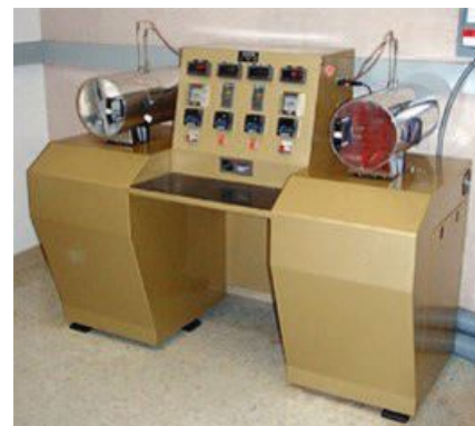
Machine used by DuPont to test ball bearing grease for more than 5,000 hours.
